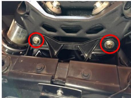
2. Next, remove the two 10mm bolts at the front of the shock mount holding the radiator support on. This will require a 10mm socket and a 10mm wrench behind the shock tower.
